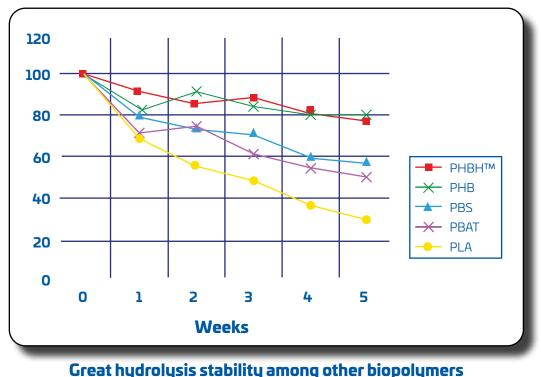
Tests were performed on Resin Powder
